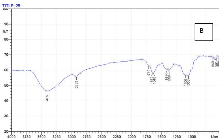
Fig. 6. FTIR spectra of seed extract (control) (A) and silver nanoparticles (B) synthesized using seed extract of B. nigra L.
